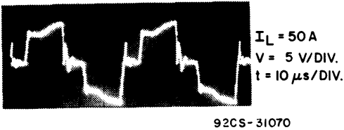
Fig. 180 - Waveform of current-sense transformer output voltage.
